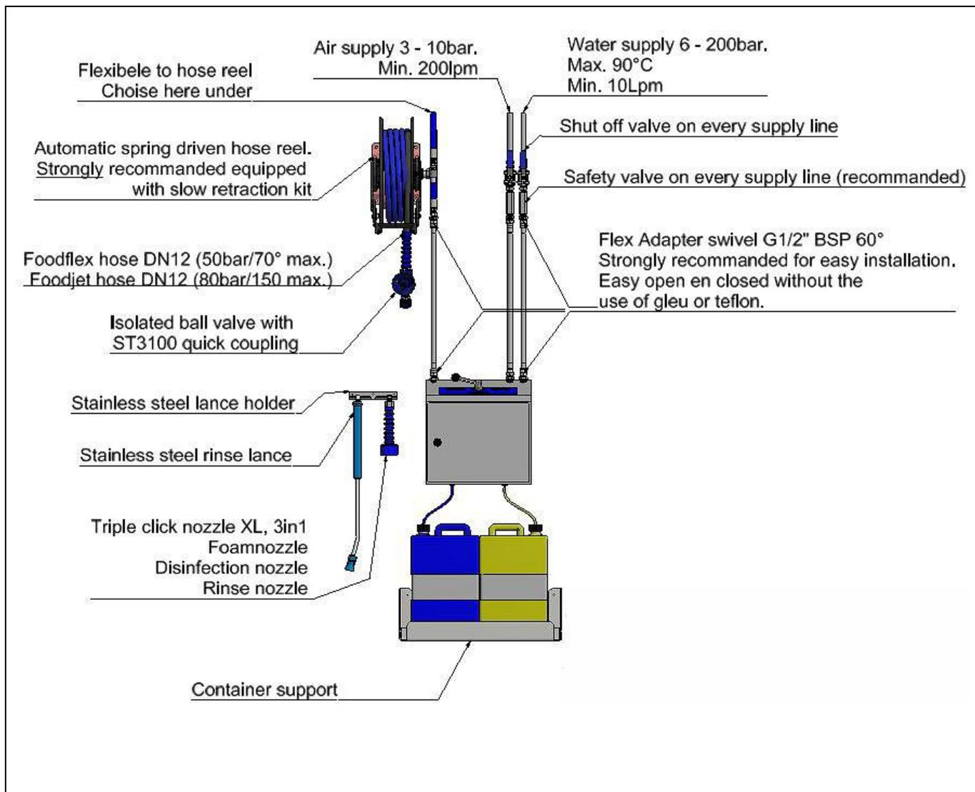
Hose lengths depend on the water pressure and water flow.
