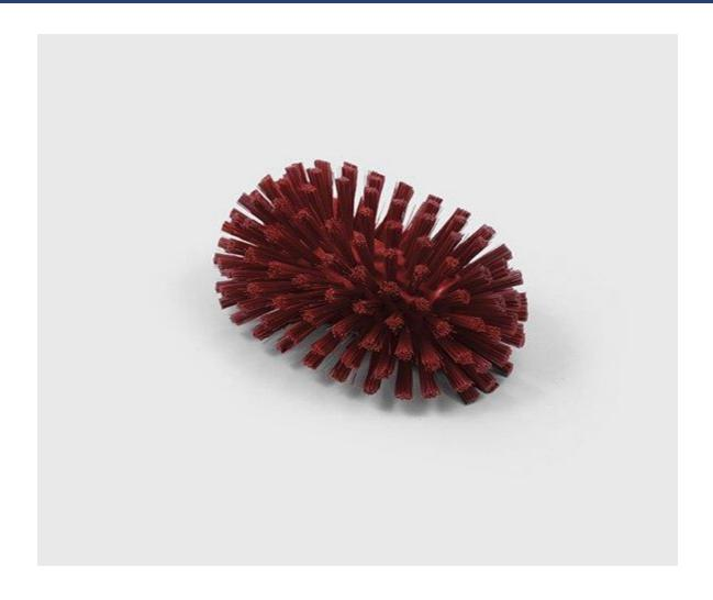
216mm overall length x 137mm wide tank brush, Polypropylene block filled medium Polyester, for cleaning tanks, vats and gullies. The material covers 360 degrees, and the only side not filled is where the handle fits. Recommended handles, ALH27 or ALH8. WFD77 is a water flow version, using the special flow through handle ALH31 and associated water flow parts. For a resin set version, see D77RES. A stiffer version is available, D79.
