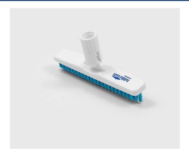
240mm grout scrub with swivel connector, filled very stiff Polyester. This brush is made to clean tile grouting. The extremely stiff material is trimmed to a V shaped point, and the universal swivel joint (the Polypropylene block is white only) allows the brush to follow the lines of grout in tiling very easily. Recommended handle, ALH7. See also ST12 for tile cleaning.
